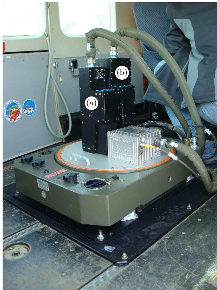
Figure 1.1: Imaging spectrometers HySpex VNIR-1600 (a) and HySpex SWIR-320m-e (b) installed on a gyro-stabilized mount in a DLR aircraft.
