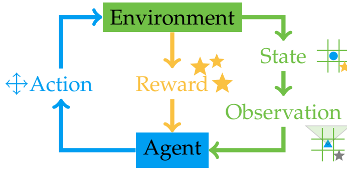
Figure 6: The optimal control setup. There is a bidirectional interaction between the agent and the environment over time.
