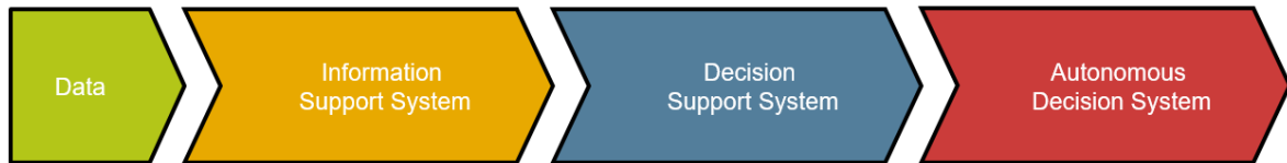
Figure 2.7: Management information systems can be differentiated into information support, decision support and autonomous decision systems based on the degrees of digital assistance they provide.
