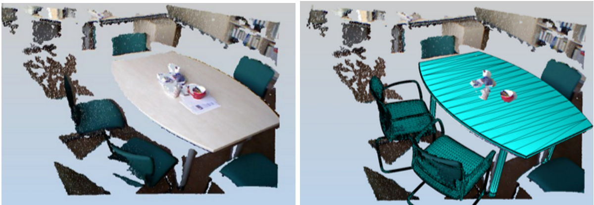
Figure 5.12: Detection of furniture instances from RGB-D data using CAD reference models as presented in [108].
