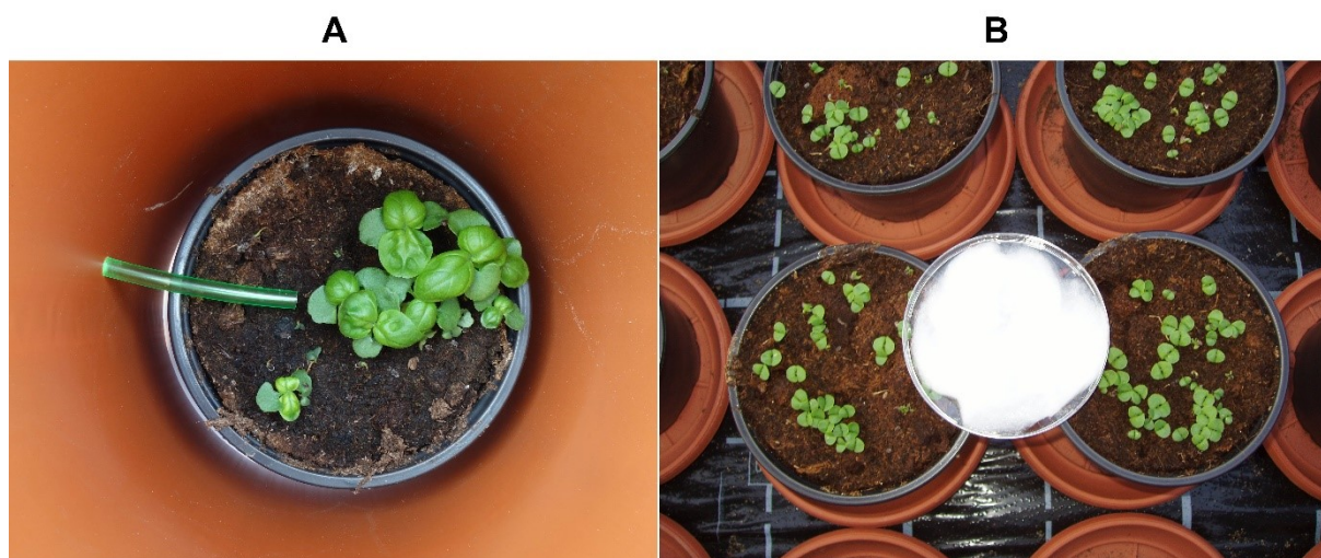
Figure 2: Ammonia sampling tube placed on the substrate surface inside the open-top chamber (A); Acid trap used as passive NH 3 samplers (plastic bowls with viscose pad) (B)
