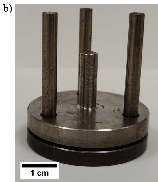
Figure 5.4: Stamping device (7). a) The MnO 2 /Ni composite stamp (8) is attached to the upper part (7a) of stamping device (7) using heat-resistant polyimide adhesive tape (4). ITO substrate (11) (not shown) is located on lower part (7b) of stamping device (7). b) Assembled stamping device. The 3 pins of lower part (7b) inserted into the holes of upper part (7a) of stamping device (7) prevent an offset during high-temperature capillary stamping.
